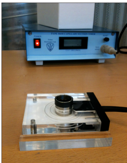
Figur 3-6 CST-analysator. Foto: Magnus Philipson, SLU.
