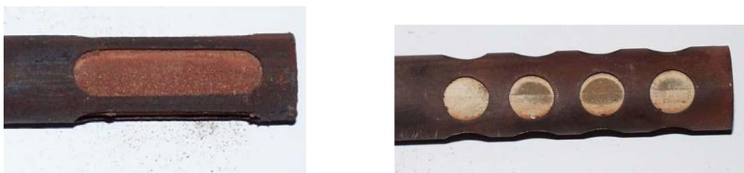
Fig. 3-4: Deposits on a sampling probe within the afterburner (left) and a deposits-free filter probe in the riser (right).
