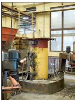
Figur 4.3 Form lyft ur vibrationsmaskin, Meag
