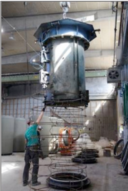
Figur 3.8 Armering placeras i form, S:t Eriks
